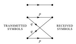
Fig. 11—Example of a discrete channel.
