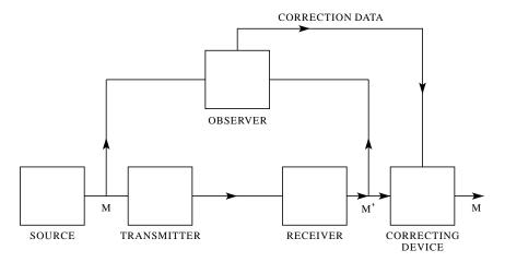
Fig. 8—Schematic diagram of a correction system.
